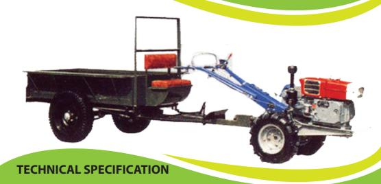
1.5 Ton Capacity Trailer 6.16 Ft body length 3.5 Ft Width 1.32 Ft Door hight 2mm thk sheet Dia50mm Round axle With Monoblack hub assembly (with brakes) 30209 Bearings 6.00x16(PRS make) tyrs Mig Mag Co2 welding Synthetic Enamel paint on the outside & Inside Coating and fitted with all Standard.
